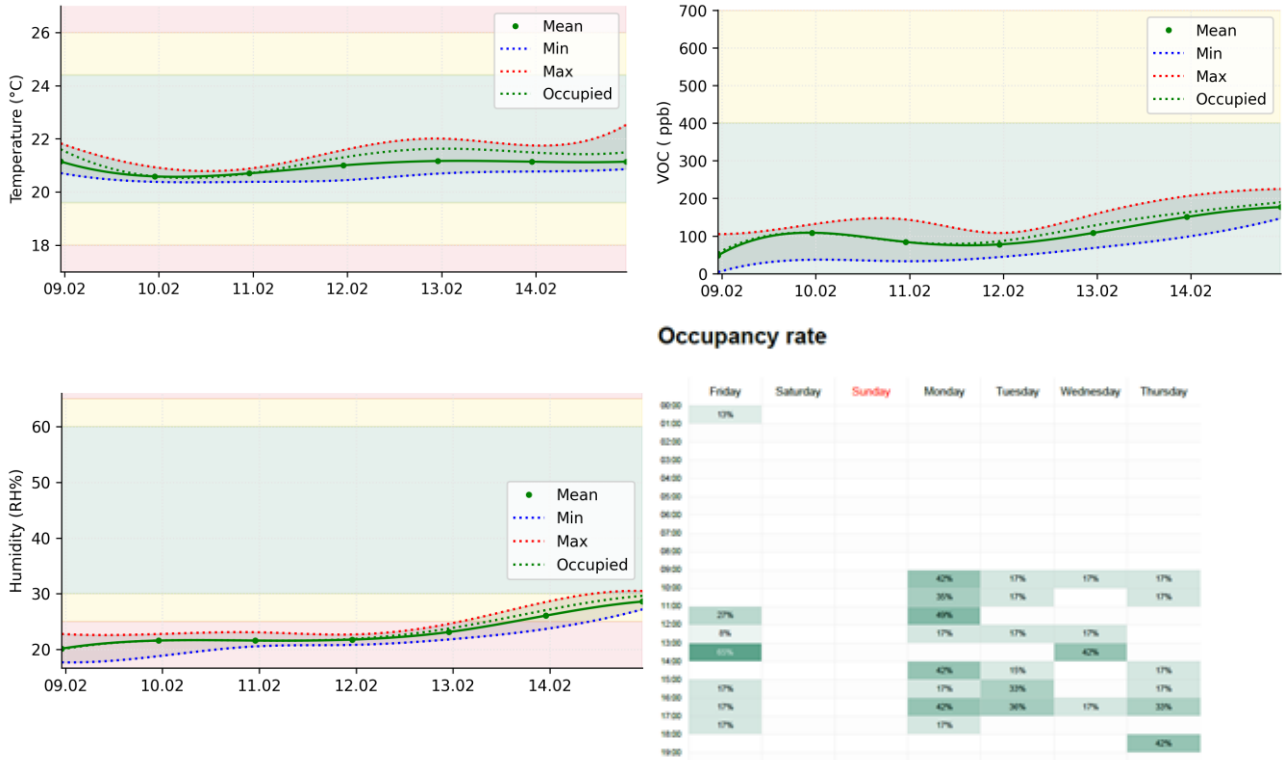
Figure 21. Graphical evolution of some of the indoor air quality parameters measured with IoT monitors for one week in February 2024 in an office at UiA in Grimstad (generated with IoT platform: roomalyzer.com).
