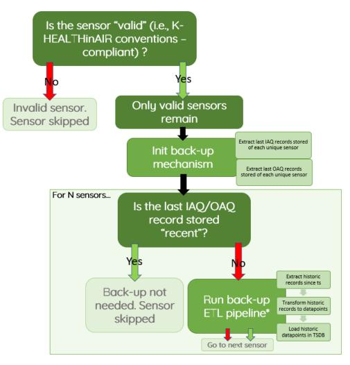
Figure 4: AQDR back-up mechanism schema. (\*) For each pipeline separately (IAQ/OAQ).
