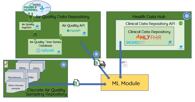
Figure 1: K-HEALTHinAIR Open Access Platform main architecture.
