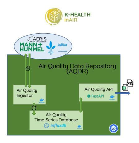
Figure 2: AQDR basic architecture (AQDR DB, AQDR Ingestor, AQDR API).
