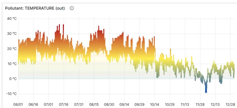
Figure 85. Outdoor temperature data (°C) provided by Aerisweather platform in the German canteens between June and December 2023 (generated with K-HEALTHinAIR platform).
